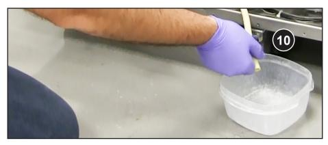
Let print material drain from hose into the drip container
