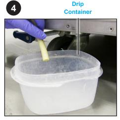
Place hose over drip container to catch any excess print material
