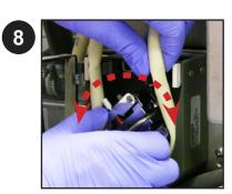
Turn mechanism to remove hose
