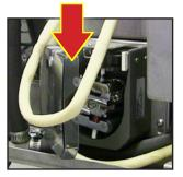
8. Remove the upper part of the hose from the connector and hold it in a vertical position (9). Stretch the hose to its full length. Let the print material drain from the hose into the drip container (10).
