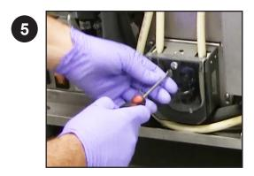
Remove cover with flathead screwdriver
