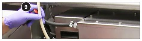
Remove top of hose from connector and hold vertically
