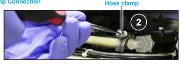
4. With a drip container and paper towels ready, pull the bottom hose loose from the connector (3) and position the hose over the container (4).
